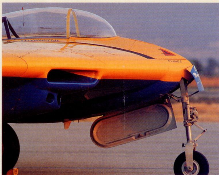
To provide the nose gear with room to retract into the aircraft's structure, the N9M's control yoke was mounted to the side of the cockpit. It was the first aircraft with fully hydraulic controls and artificial feedback.
